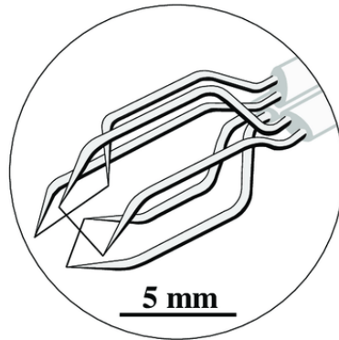
Figure 1.24 General 3-dimensional wire probe [27]
